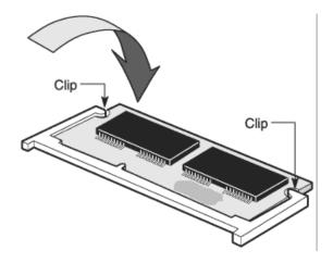
Figure 41. SODIMM Installation – Rotating the Module Downward
